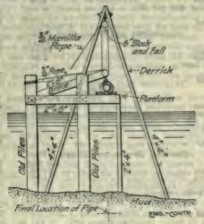
Fig. 13.-Laying Subaqueous Pipe Line.
